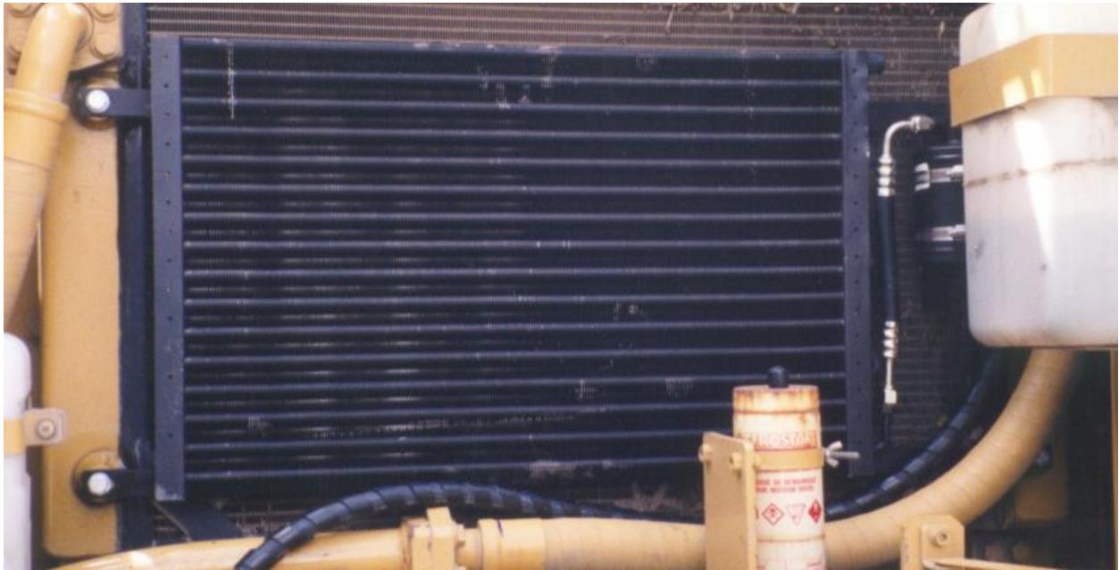
Condenser in place with attached drier and hoses.
